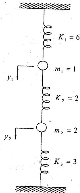
(1) Please derive the system of two second order differential equations governing the position of the weights relative to their equilibrium positions at any time  $t = 0$ . Note that only the system of differential equation is required. (5%)
